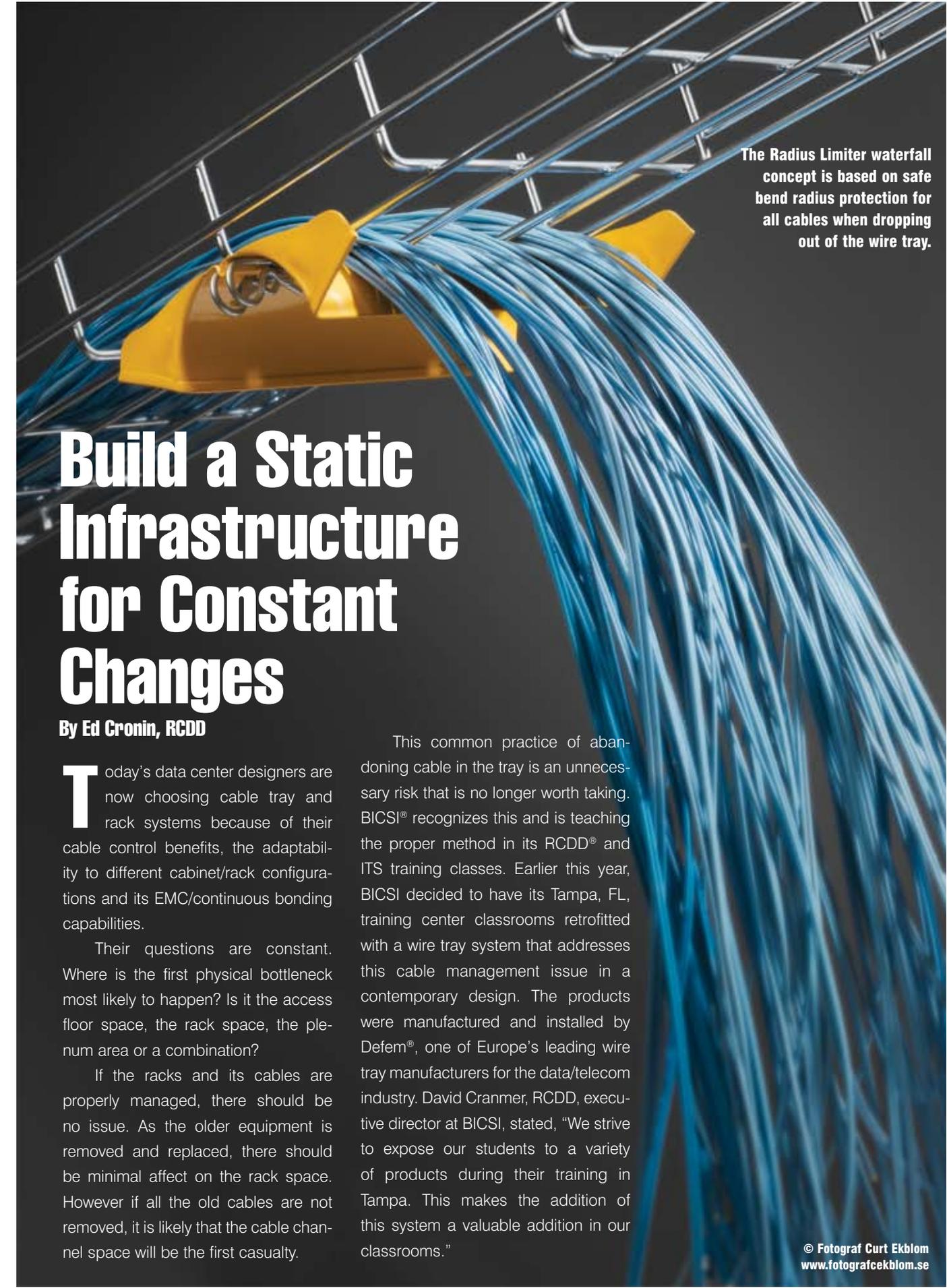
The Radius Limiter waterfall concept is based on safe bend radius protection for all cables when dropping out of the wire tray.
